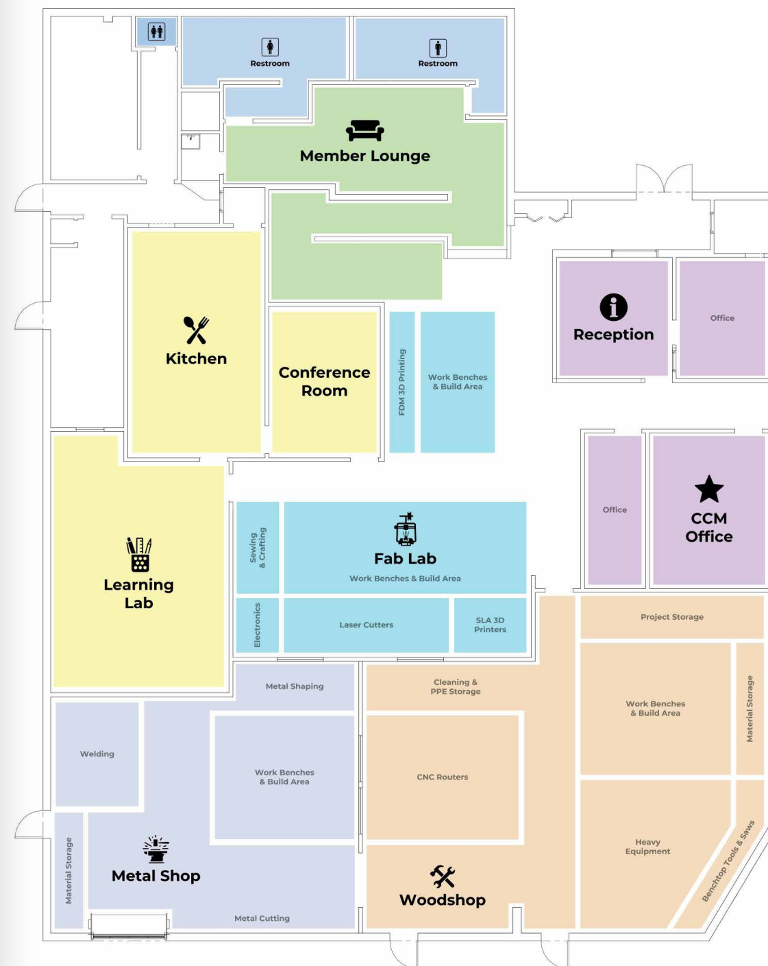
CCM FLOOR PLAN - EQUIPMENT LAYOUT
