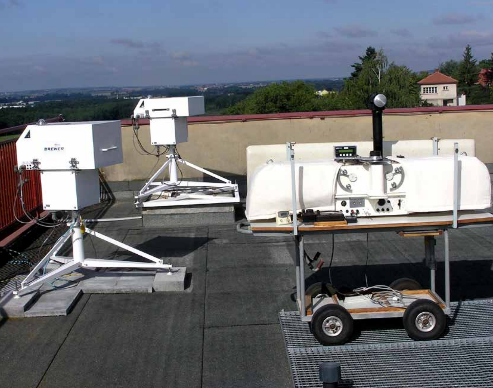
▲ Dobsonian spectrophotometer D074 (right) and Brewer spectrophotometers B098 and B184 (left) in Hradec Králové.
