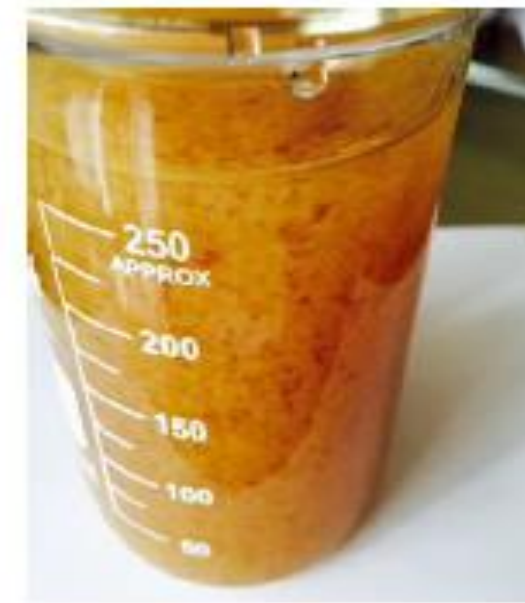
Coagulation of the leachate water after the EEC system treatment
